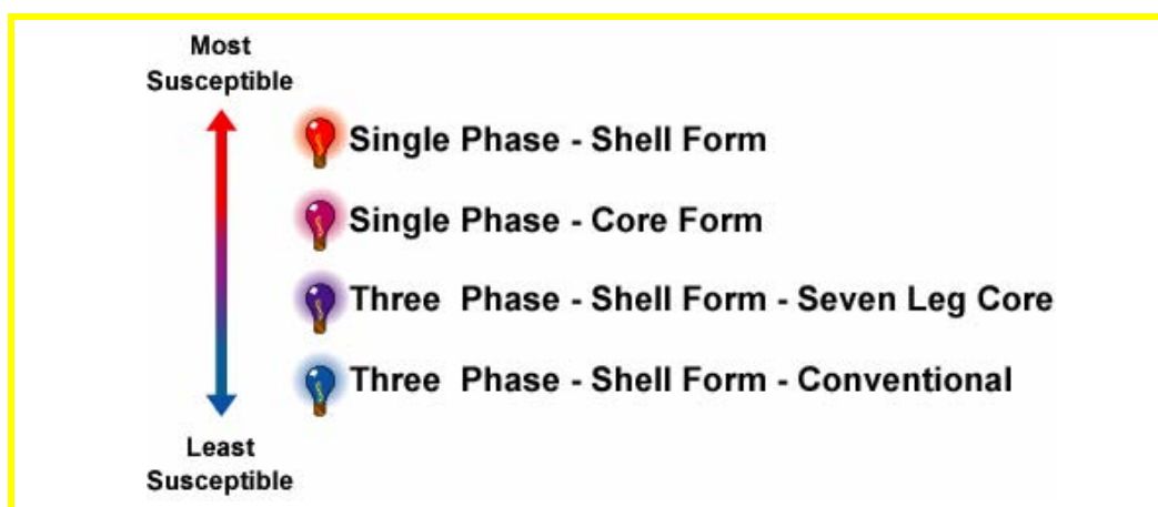
Figure 9-42 Transformer Susceptibility to GIC Induced Saturation
